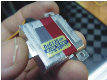
Insert the servo into the frame and attach with screws (flap servo MKS612 **Glider** only 2 screws). Set the servo travel to neutral position by servotester.
