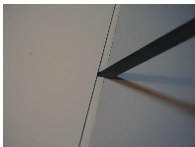
4. Under servo make the surface ragged
