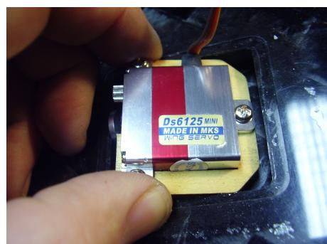
15. Move rolldrive 20° in the direction of aileron, slide it on servo shaft and fix with worm. Aileron in **NEUTRAL** position !
